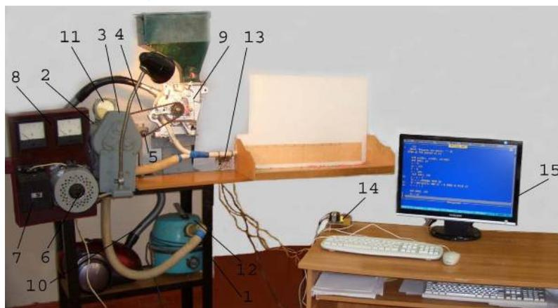
Fig. 5. **Laboratory installation:** 1 – frame; 2 – electric motor; 3 – reducer; 4 – chain; 5 – tension roller; 6 – voltage regulator; 7 – current rectifier; 8 – shield with control devices; 9 – seeder; 10 – vacuum unit; 11 – diaphragm thimble Tm MP-100; 12 – air-inflating device with adjustable air supply; 13 – sensors for measuring of seed speed; 14 – control unit; 15 – personal computer
