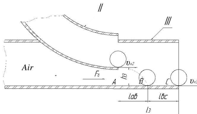
Fig. 4. Scheme of movement of the seed on the drill tube area III
