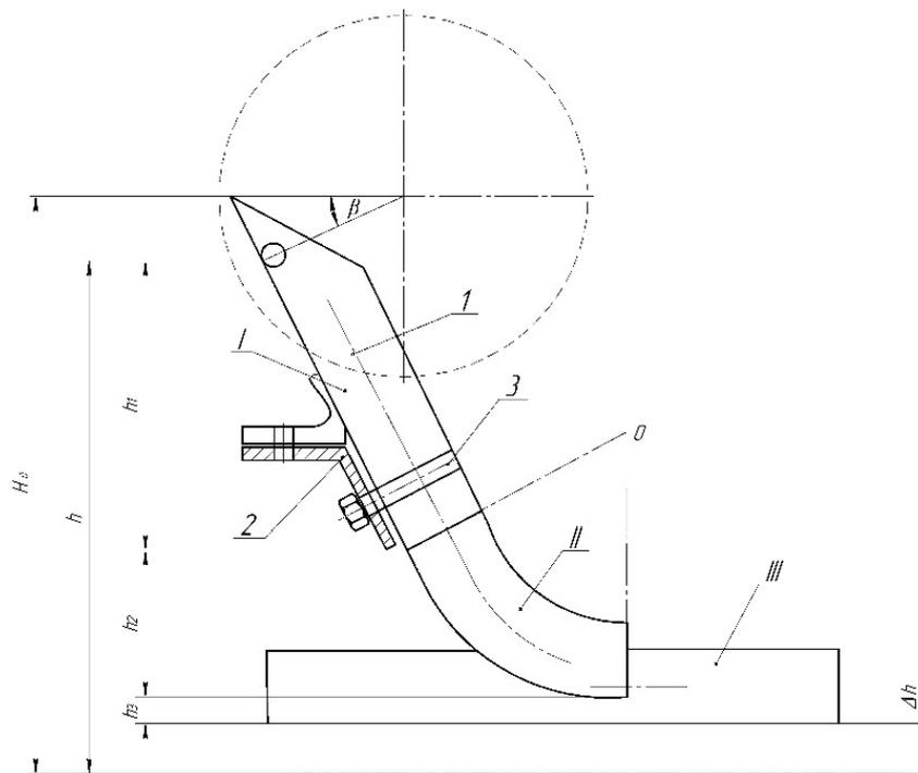
Fig. 1. Scheme of drill tube of pneumatic drill
