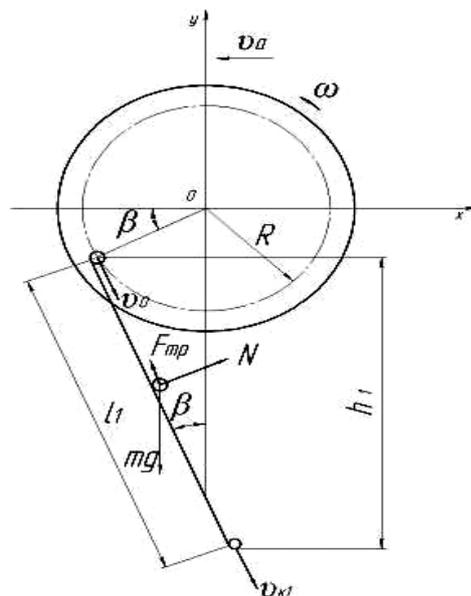
Fig. 2. Scheme of movement of the seed on the drill tube area I
