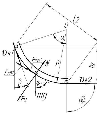
Fig. 3. Scheme of movement of the seed on the drill tube area II
